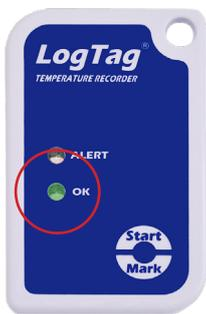
Check that the green OK LED light is flashing green.
