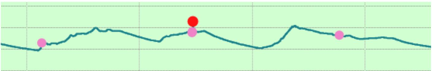
A section of a results graph showing the pink Inspection marks (made when the MARK button is pushed) and a red Download mark (created automatically when the data is downloaded).
