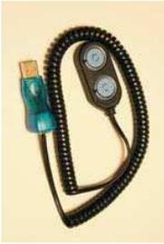
The reader is the cable that was supplied in the kit. It will typically be a USB device at one end and either a double blue circle or a 45° angled connector at the other.
