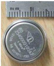
The logger is the small “watch battery” looking device that may be on a plastic holder.
