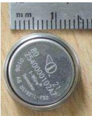
The logger is the small “watch battery” looking device that may be on a plastic holder.
