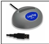
A reader (also known as a cable adaptor) is required to connect the Logtag to the PC. The reader has a USB connector for your PC
